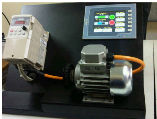
VARIABLE SPEED DRIVE WITH BUILT IN LOGIC CONTROLLER & TOUCH SCREEN, VERY ECONOMIC AND DOES AWAY WITH NEED FOR SEPARATE SMART RELAY
